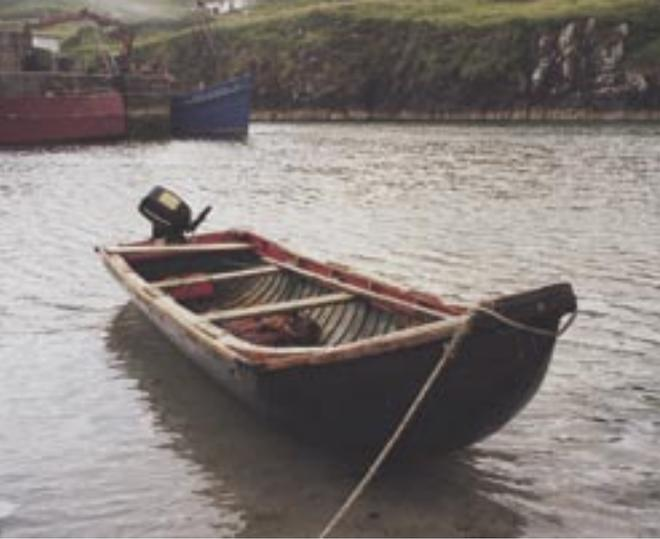
**Figure 7.** Inishturk Island curragh, fibreglass covered, 2001.
